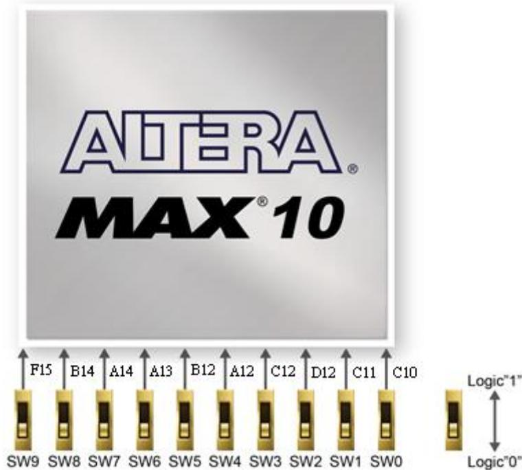
**Figure 3-15** Connections between the slide switches and MAX 10 FPGA
