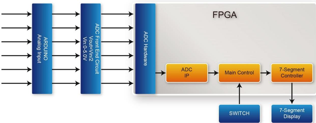
**Figure 5-9** Block diagram of the ADC measurement demonstration
