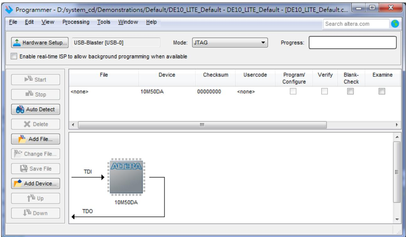
**Figure 3-6 FPGA detected in Quartus II programmer**
