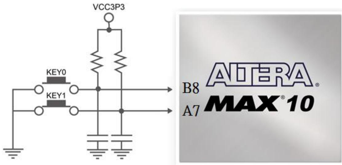
**Figure 3-13** Connections between the push-button and MAX 10 FPGA
