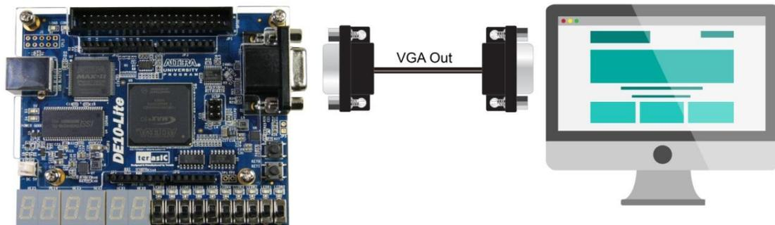
Figure 5-7 The setup for the VGA Pattern demonstration
