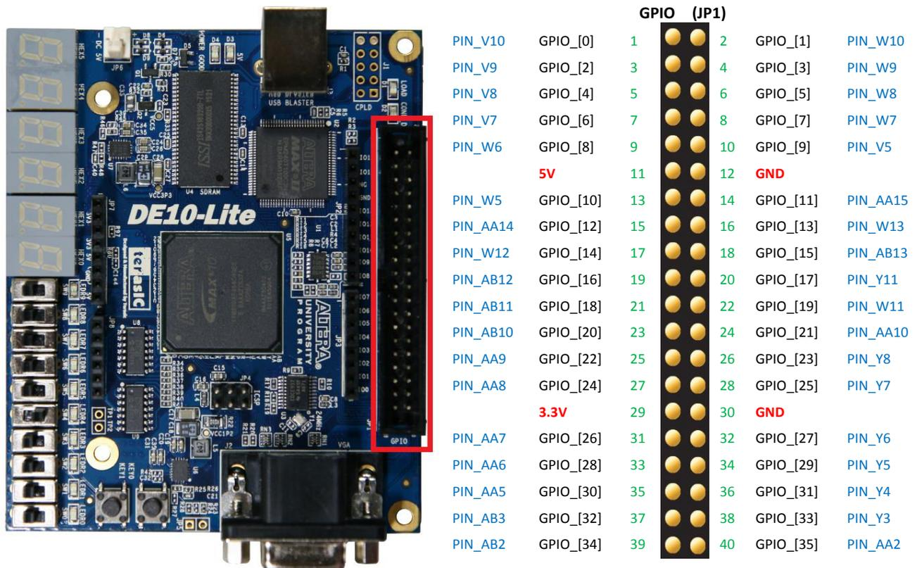
Figure 3-18 I/O distribution of the expansion headers
