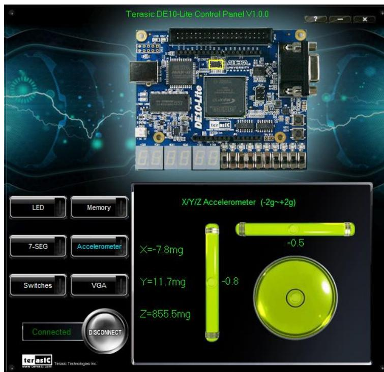
Figure 2-7 Level by G-Sensor
