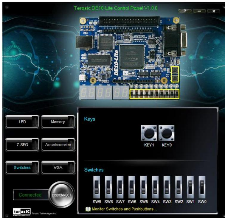
**Figure 2-5 Monitoring switches and buttons**
