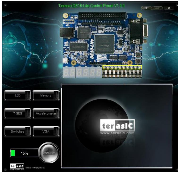
**Figure 2-1 The DE10-Lite Control Panel**
