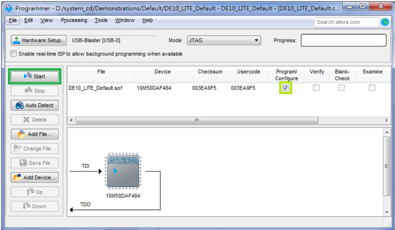
**Figure 3-9 Program .sof file into the FPGA device**
