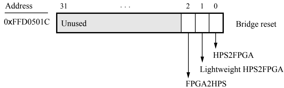
Figure 5. FPGA bridge reset register.
